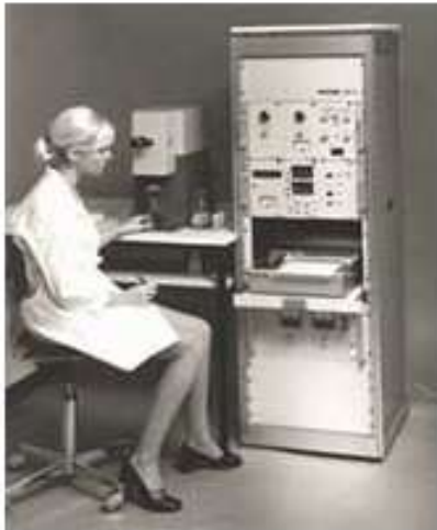
ICP 11 (1969) Distributed by Phywe, Göttingen The first commercial flow cytometer PDP 11 computer
