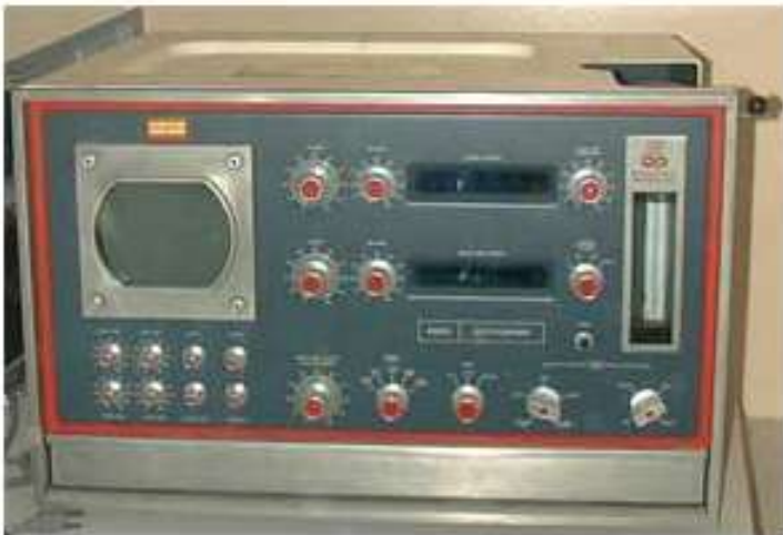
ICP 11 (1969) Distributed by Phywe, Göttingen The first commercial flow cytometer PDP 11 computer
